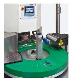
Multifunction jig surrounded by pad printing machine and components
